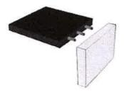
The doweled joint is merely a butt joint that uses wooden dowels (A dowel is a solid cylindrical rod, usually made of wood) to help align and strengthen the bond between two boards. Often times a doweled joint is made into a very visually appealing joint by passing the dowels completely through the side piece allowing them to show through and sanding them flush with the surface. A well-made dowel joint is as strong as a mortise
