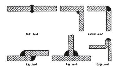
BASIC TYPES OF WELDED JOINTS
