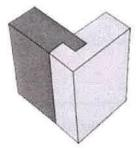
Rebate and Dado joints are simple joints that create an incredibly strong bond by inserting one piece of wood, a reabte, into a groove, a Dado, in another piece of wood. In addition to increasing the glue surface, the rabbet also provides support and alignment for the two adjoining pieces. This joint is the backbone of cabinet box and bookcase construction. Just about any variation of this joint can be cut with either a table saw (with dado blade) and/or a router (with dado jig).
