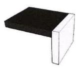
The butt joint is the simplest but also the weakest type of joint. It is created by simply butting two boards together (hence the name) and attaching them using glue or with a nail or screw for extra strength. This joinery application is usually used to glue narrow boards side to side to form one wide panel, such as a cabinet door or a table top. Butt joints are not commonly used in furniture construction, due to their weaknesses and for their lack of any obvious aesthetic quality.
