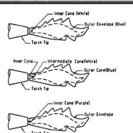
TYPES OF OXY-ACETYLENE FLAME
